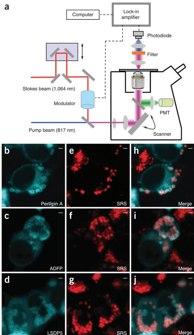
**Figure 1** | Visualization of cellular fat storage in lipid droplets using SRS microscopy. (a) Experimental scheme of label-free SRS microscopy for *in vivo* lipid imaging. PMT, photomultiplier tube. (b–d) YFP fluorescence images (b–d), SRS signals (e–g) and merged images (h–j) of HEK 293 cells expressing YFP-tagged perilipin A (b,e,h), ADFP (c,f,i) and LSDP5 (d,g,j). Scale bars, 1  $\mu$ m.
